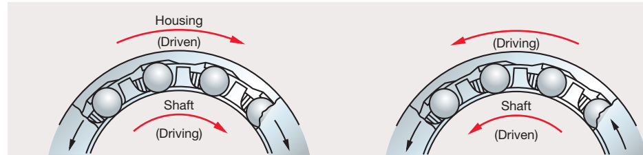
Fig. 1 When Clutch is Engaged
